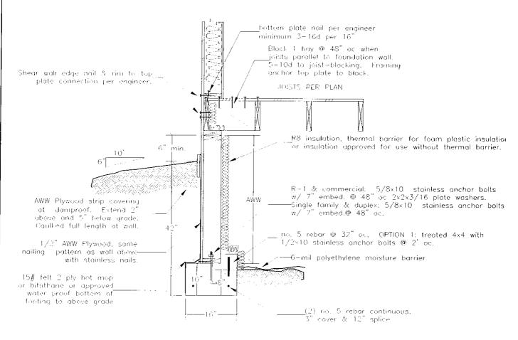
Maximum 3' differential fill between inside versus outside or engineered design required
